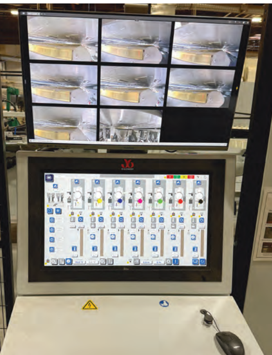
JB KomandCenter® dashboard, includes all JB product controls and displays for the InKomand, IR dryers/AutoDryer control, UV curing section and VisionMaster.
