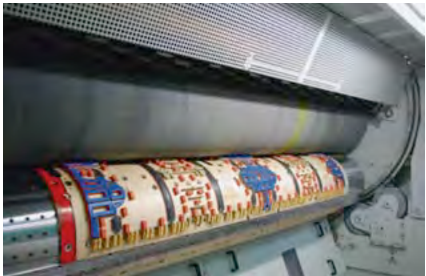
THE DUAL DIECUTTER ALLOWS THE MACHINE TO BE PRE-SET FOR THE NEXT ORDER WHILE THE CURRENT ORDER IS RUNNING.
