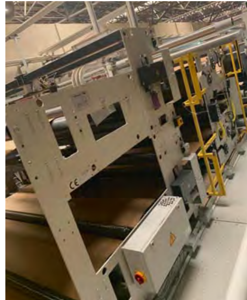
The new corrugator is equipped with E+L Corraligner
