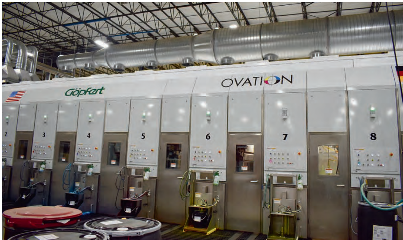
The dust collection system above the press adds additional assurance of uptime.
