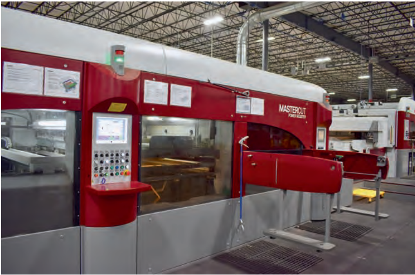
The Mastercut's power registration system ensures print to cut register accuracy.
