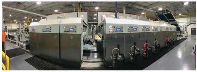
The diecutter has two top printing units and five bottom printers. ColorDry™ XL3000 IR dryers are located after each print station.
