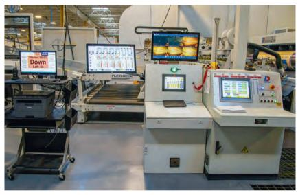
JB Machinery's new KomandCenter<sup>™</sup> system provides one central dashboard for real-time operator monitoring.
