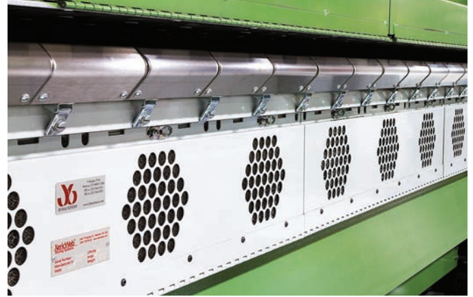
All four print stations on the Hycorr 7590 VO are equipped with JB Machinery dryers. The first also has the JB Kleenplate Wash Eliminator.
