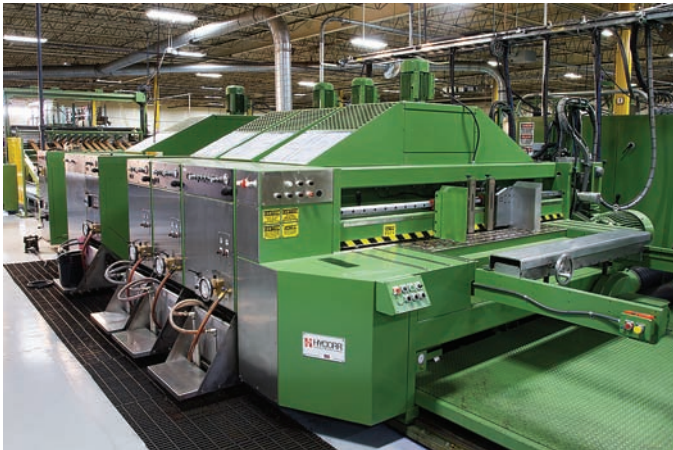
Hycorr’s 7590 VO 66-inch by 115-inch four-color rotary diecutter is equipped with a Hycorr lead edge feeder with a vacuum sheet cleaner.
