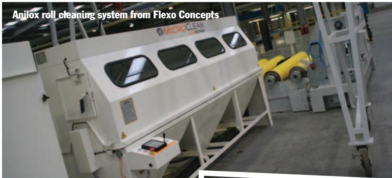
the system's operational cost is low, and there is virtually no waste material that needs to be disposed of. MicroClean is also a fully automated system; once the operator has loaded the roll in the machine, he merely selects the cleaning programme, hits the button and walks away. When the cleaning cycle is complete, the roll is press-ready.
