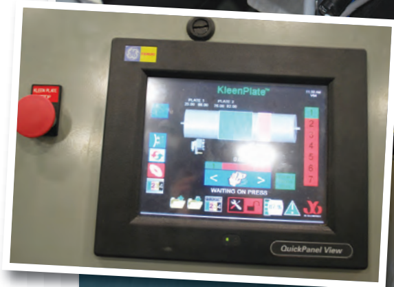
TOP: THE LINT-FREE CLOTH REMOVES A PRECISE LAMINAR FILM OF INK FROM THE PLATE AFTER THE INK HAS BEEN TRANSFERRED TO THE SHEET. ABOVE: THE PRESS OPERATORS CAN SET UP, CONTROL AND MONITOR THE SYSTEM THROUGH A USER-FRIENDLY TOUCH SCREEN CONTROL.
