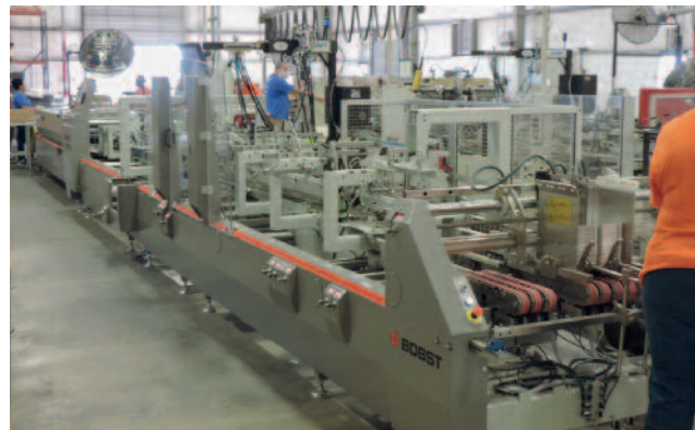
AMONG THE CARTON PLANT'S FINISHING EQUIPMENT IS A BOBST EXPERTFOLD.
