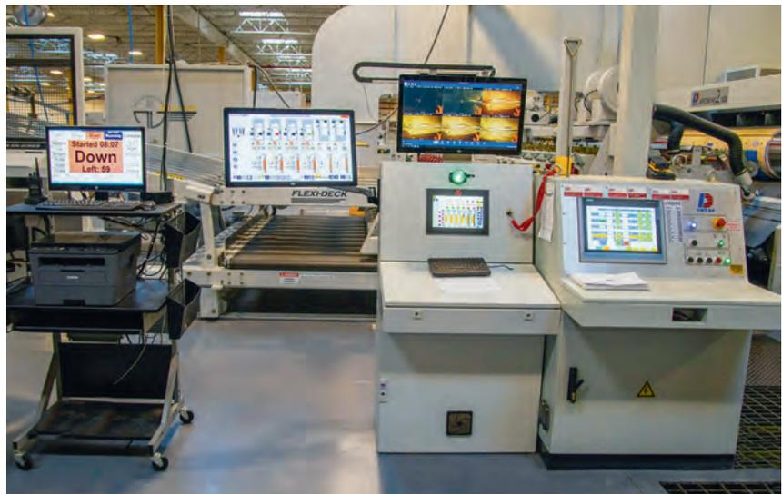
JB Machinery's new KomandCenter™ system provides one central dashboard for real-time operator monitoring.
