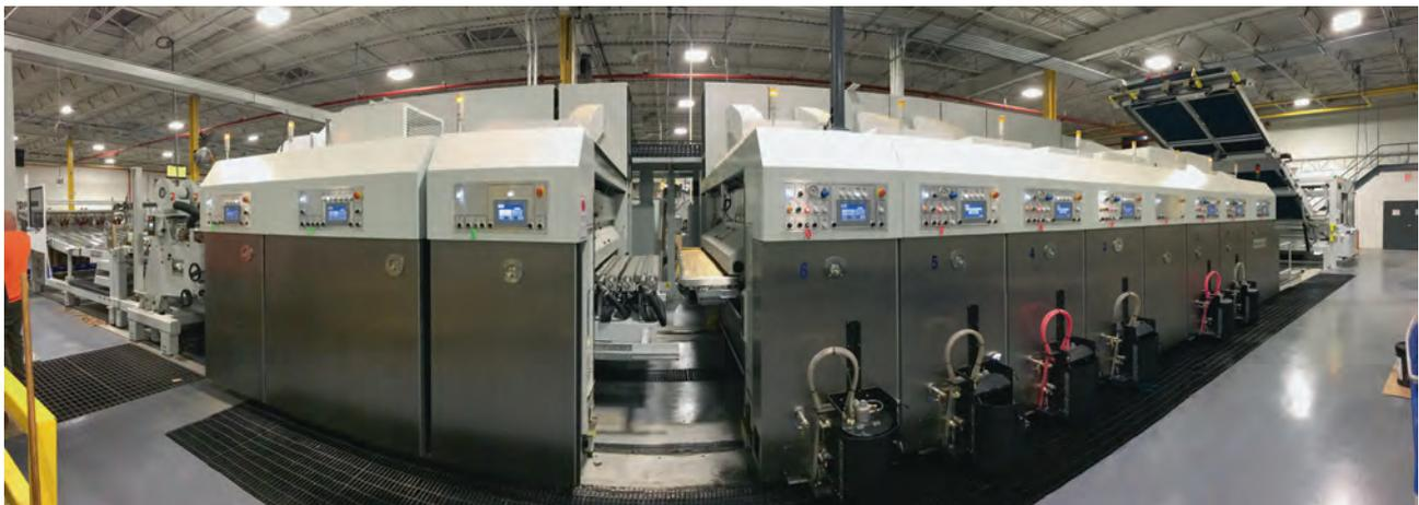
The diecutter has two top printing units and five bottom printers. ColorDry™ XL3000 IR dryers are located after each print station.
